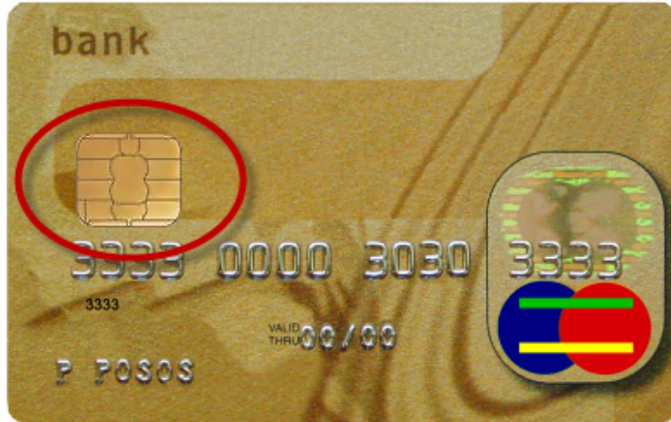
FIGURE 6 – AN ILLUSTRATION OF AN ISO 7816 CHIP PLACED IN A PAYMENT CARD (Source: http://en.wikipedia.org/wiki/File:Smartcard2.png licensed under Creative Common Share Alike)
